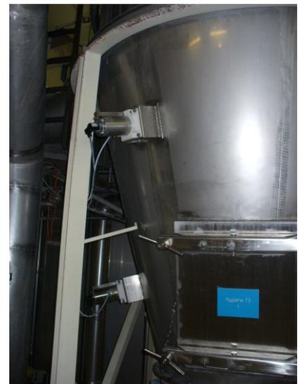
Picture right: example two mounted pneumatic impactors
